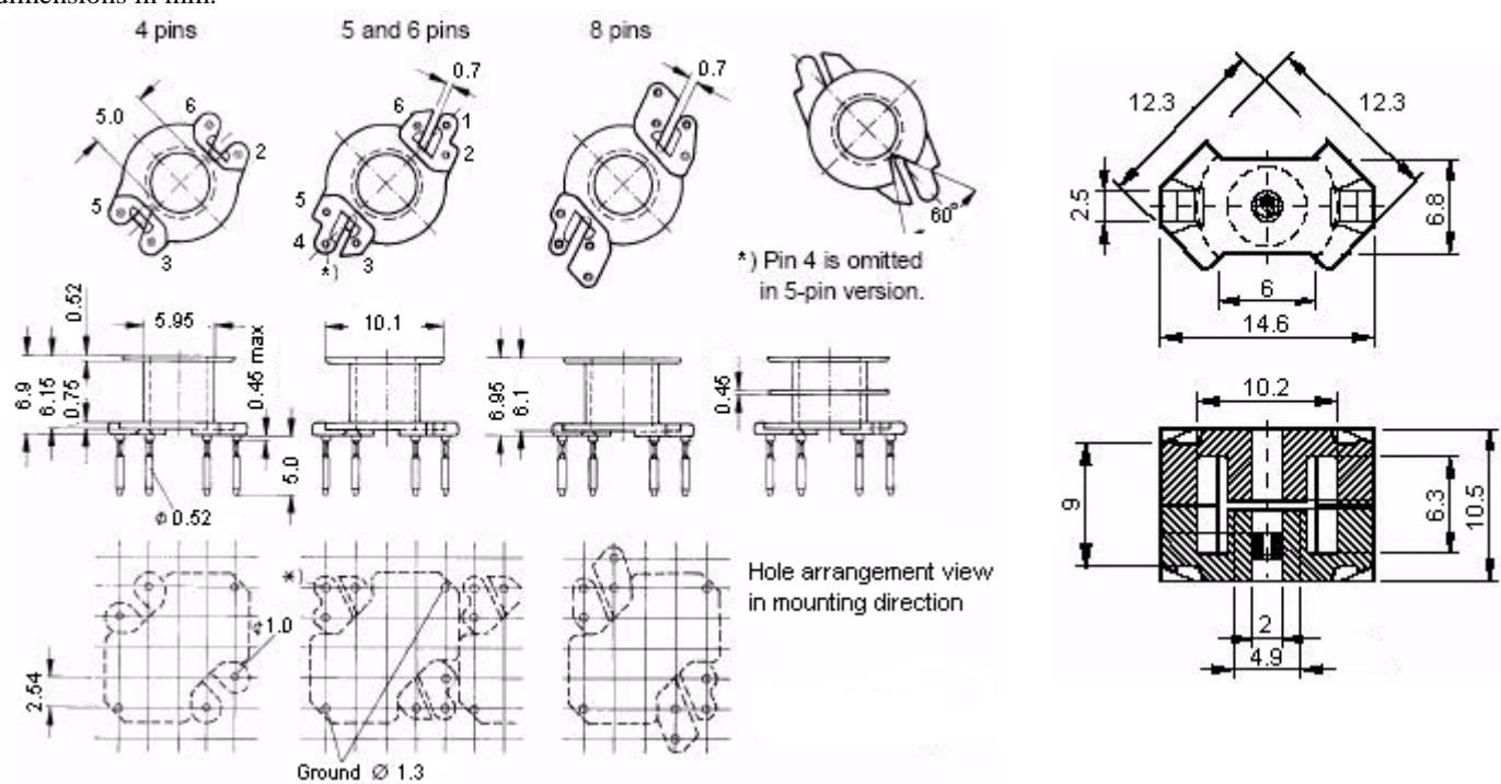
**Other versions available:** RM5 low profile coilformer & cores & RM5 low profile SMD coilformer.
